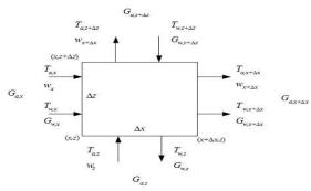
Figure 1: Elementary cross-section through a fill region of a rectangular cooling tower (3)
